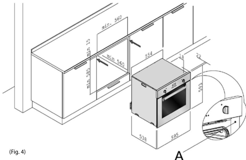
3. Put the unit on the edge of the cabinet and run the power cord through the rear wall of the cabinet so that its plug is accessible after installation.
